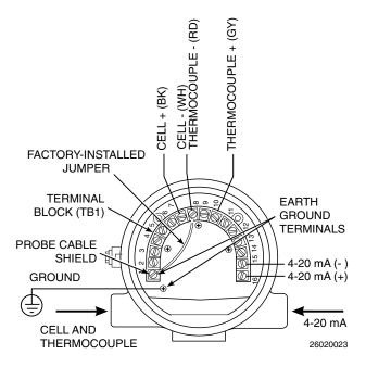
Figure 6-4. Model 3081 Transmitter Terminal Block
